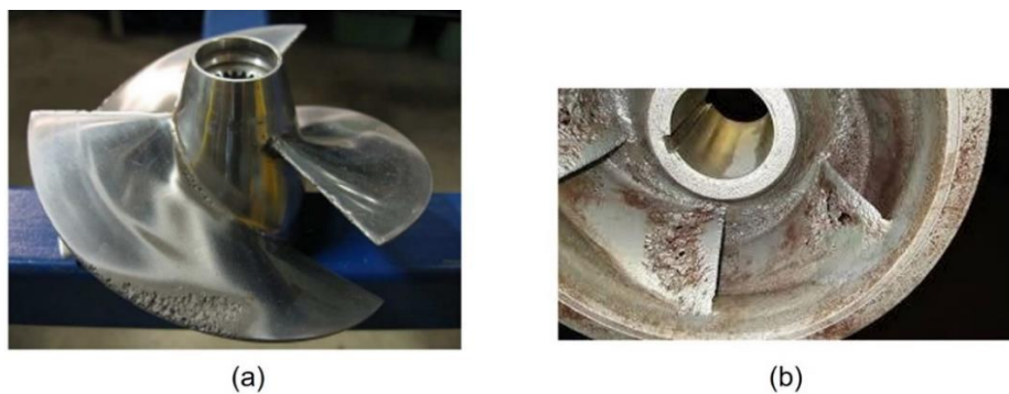
Fig. 1.7: Damage due to cavitation (a) erosion near the tip of propeller blade (Britannica), (b) centrifugal pump impeller (Noon et al. 2021).
